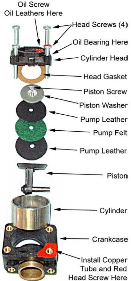
7. Insert the copper tubing between the pump head and block, into the holes that have been reamed for this purpose. Insert the red screw through the copper tubing. Insert the other corner screws and tighten all securely. Avoid excessive tightening of these screws as this may distort the main bearing of the pump, causing hard turning and overheating.
