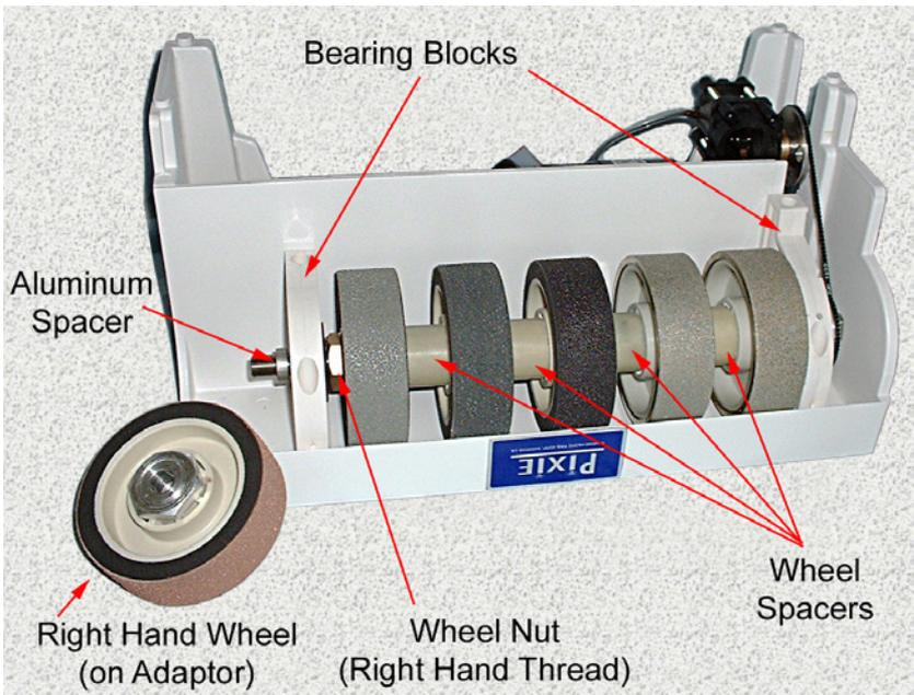
left Galaxy wheel and the outer side of the housing. The guard was attached to the left bearing block. This bearing block, and the similar right bearing block must both be removed by unscrewing the two socket-head screws that attach each block to the housing. An allen wrench (3/16 inch) must be used. Once the two bearing blocks are free, the wheel and shaft assembly can be moved to allow the two belts to be slipped off, and the wheel assembly can then be lifted out.
