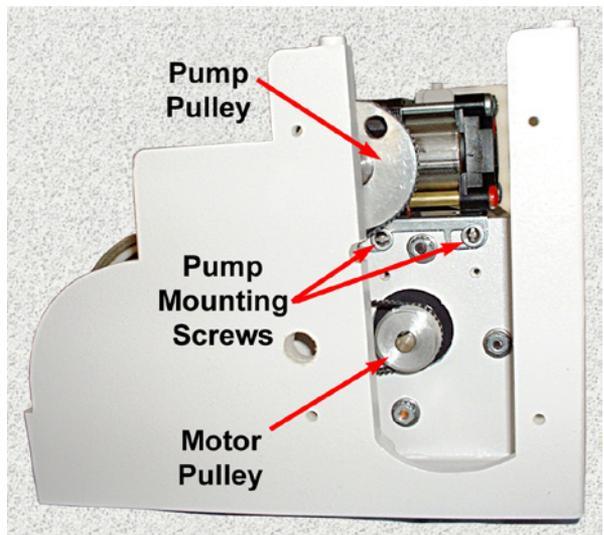
4. The four corner screws in the pump are to be removed next, but note the position of the red corner screw as it and its copper tubing sheath must be returned to its proper corner when the pump is reassembled.
