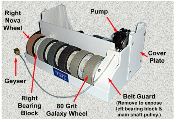
3. Remove the two screws attaching the pump bracket to the housing. Once the pump is detached from the housing, remove the bracket from the pump.
