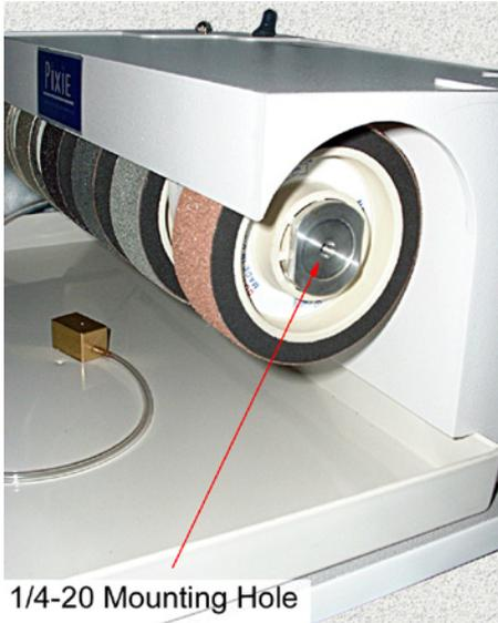
1. Thread the Nova Disc into the 1/4-20 mounting hole in the right end of the machine.
